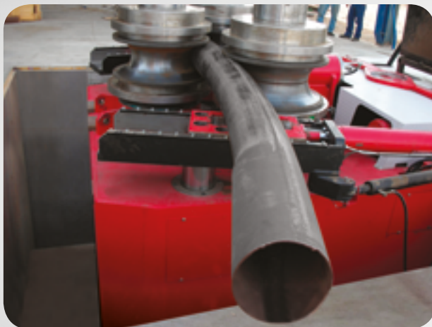
MCP 26 TUBE 324 mm
